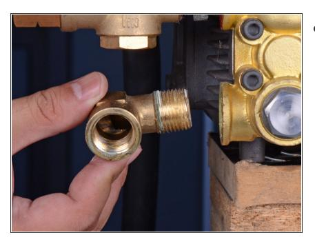
Remove the input elbow fitting.
