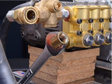
Use a 1" or large adjustable wrench to loosen and unscrew the pump input elbow.
