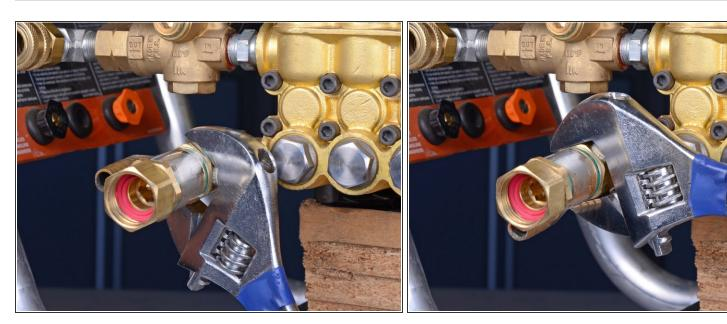
Use a large adjustable wrench to loosen and unscrew the filter.
