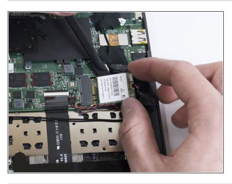
Remove the WiFi card from the motherboard by sliding it out at an angle.
