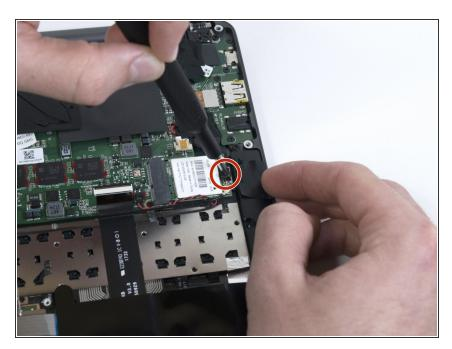
Use a Phillips #00 screwdriver to remove the single, 2 mm screw from the WiFi card.
