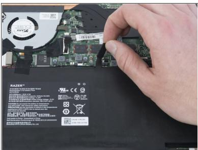
Use your fingernail to pry up and disconnect the battery from the motherboard.
