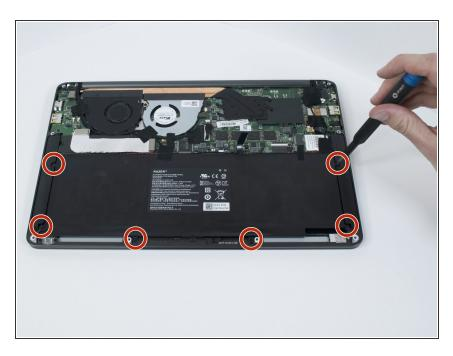
Use a Phillips #00 screwdriver to remove the six, 5mm screws securing the battery.
