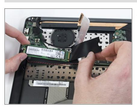
Remove the SSD from the motherboard by sliding it out at an angle.
