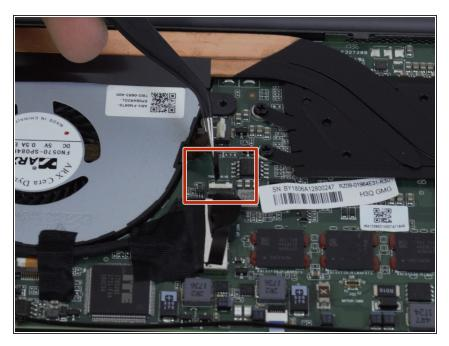
Use tweezers to pull the fan cable out of the opened connector terminal.
