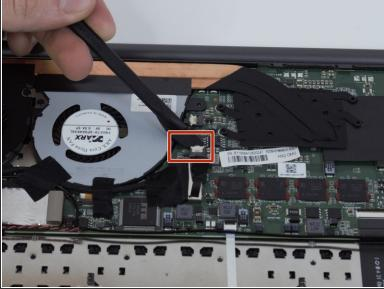
• Use a plastic spudger to lift the white clasp on the fan connector.
