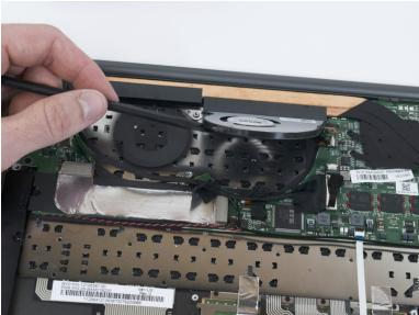
Use a plastic spudger to slide the fans out of the case.
