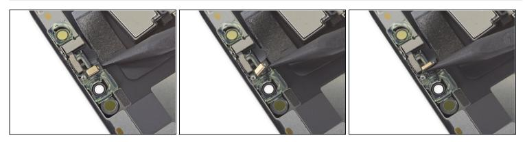
• Use the point of a spudger to lift and separate the microphone from its notch in the front panel.
