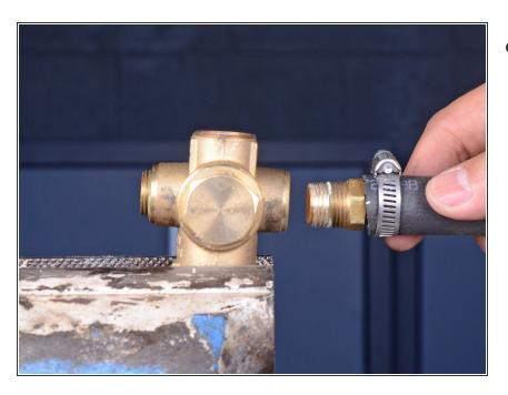
Remove the return hose nipple with the hose attached.
