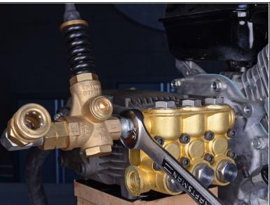
• Use a 3/4" or adjustable wrench to loosen and disconnect the coupling from the pump assembly.
