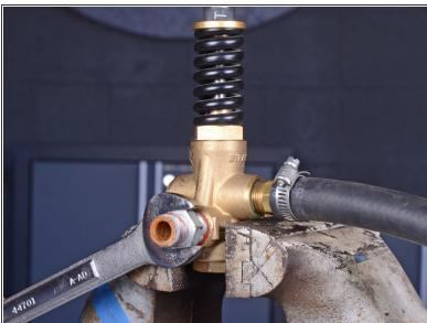
• Use a 3/4" or adjustable wrench to loosen and unscrew the coupling nipple from the unloader.
