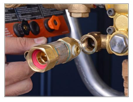
Remove the filter with the return elbow attached.
