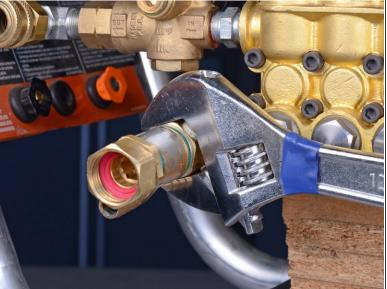
Use a large adjustable wrench to loosen and unscrew the filter.
