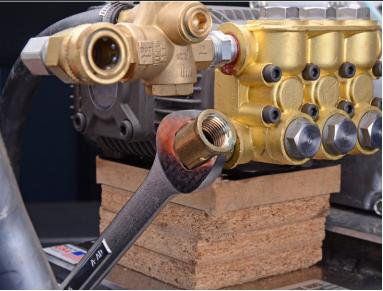
Use a 1" or large adjustable wrench to loosen and unscrew the pump input elbow.
