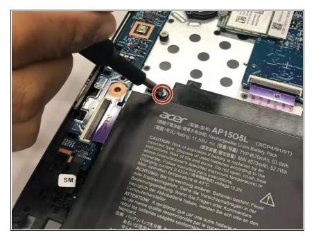
Remove two 4 mm screws at the two corners of the battery using the Phillips #1 screwdriver.
