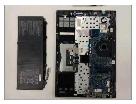
Remove the battery from the device.
