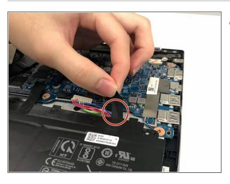
Carefully remove the three tapes on the battery.
