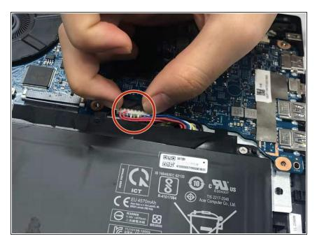
Carefully slide the battery connector out of its motherboard socket.
