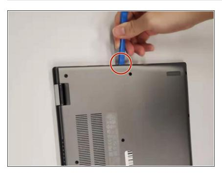
Use an opening tool to pry the back cover open.
