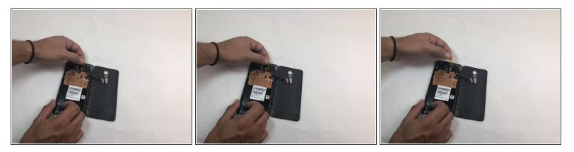
• Remove the opaque yellow sticker that indicates where the fingerprint scanner is connected to the back of the device.
