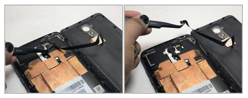
• Use the tweezers to pull at the base of the film to remove the fingerprint scanner.
