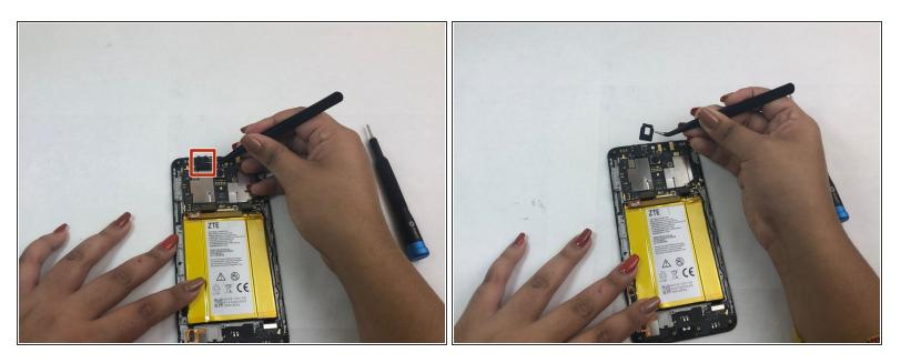
Use tweezers to remove the protective foam surrounding the headphone jack at the top left of the device.
