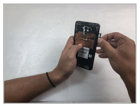
• Remove the SD and SIM cards by pulling out the card tray from the slot on the right side of the device.
