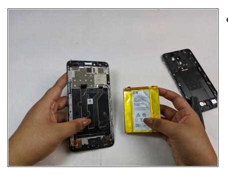
The LCD and its frame are now free to be replaced with a new component.
