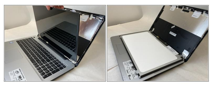
• Using your hands, carefully lift the screen from its housing and lay it flat on the keyboard.
