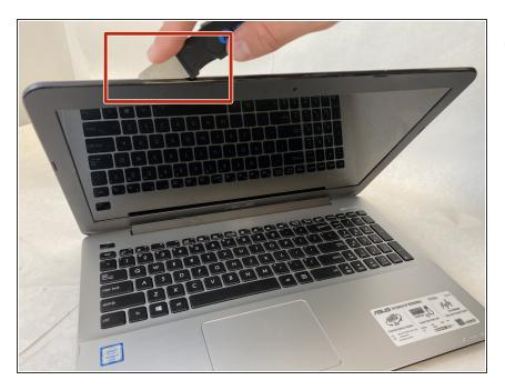
Use a Jimmy to separate the outer panel of the monitor from the bezel. This is accomplished by wedging the tool in the small crease and pulling apart.
