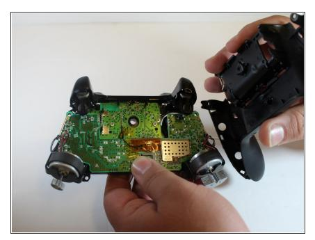
Remove the back cover of the controller using the spudger.
