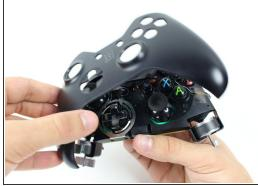
Remove the front cover of the controller. using the spudger.
