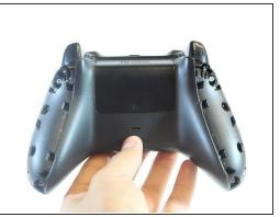
Remove the side handles with the iFixit plastic opening tool by wedging it around the seam of the handles.
