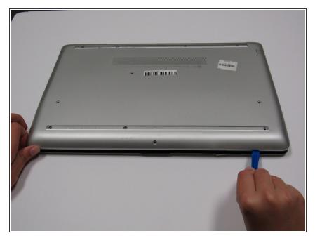
Close the screen and flip over the laptop. Using the plastic opening tools, gently take off the back cover starting from the middle, bottom edge.
