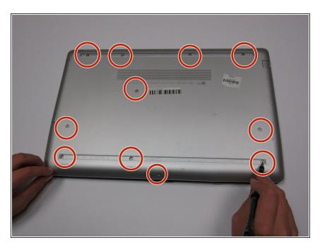
Using the Phillips #1 screwdriver, unscrew the eleven 9.0 mm screws holding the back cover in place.
