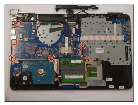
Remove the six screws from the motherboard using a Philips #0 Screwdriver.
