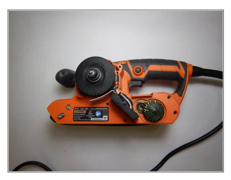
Remove the plastic housing by lifting it up from the device.
