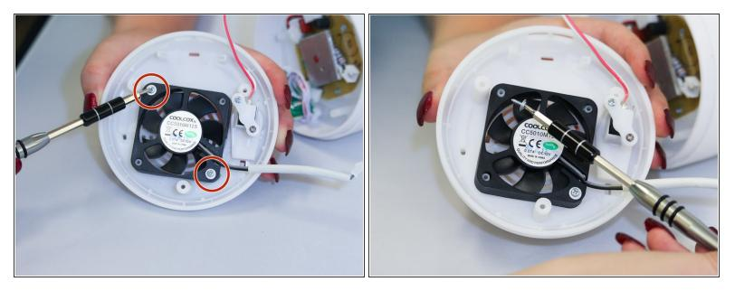
• Using the Phillips #00, remove two 10.0 mm screws holding the fan onto the base of the diffuser.
