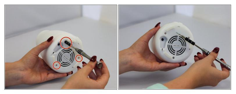
Using a Phillips #00 screwdriver from the iFixit kit, remove all three 10.0 mm screws on the bottom piece.
