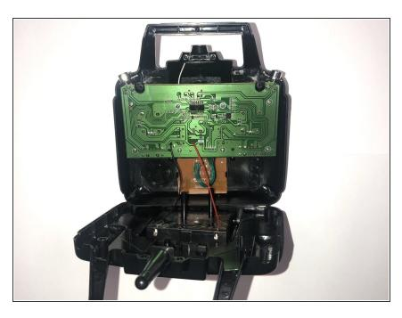
Since the battery wires are still attached, carefully move the rear panel down to expose the motherboard.
