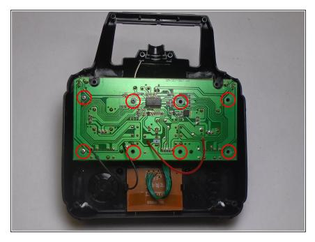
Remove the eight 5mm Phillips #1 screws from the motherboard.
