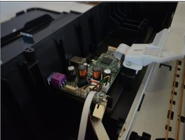
The mother board is located at the back of the printer.
