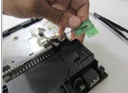
Remove the circuit boards by carefully lifting and pulling away from the device.
