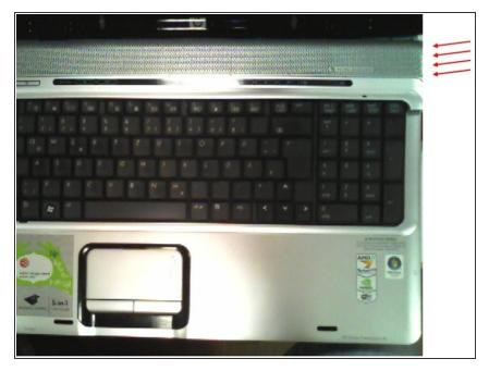
Turn laptop around and remove the plastic top shown on image. Start from the right and be careful with the flat cable in the center. Pull slowly and then remove the flat cable from its motherboard connector (see next step)
