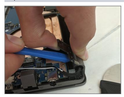
Using the opening tool, lift up the flaps that secure the screen to the base.
