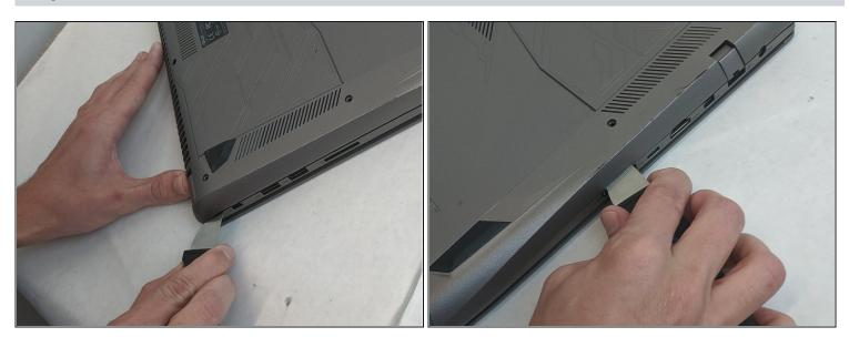
• Use a Jimmy to carefully free each side of the bottom casing.
