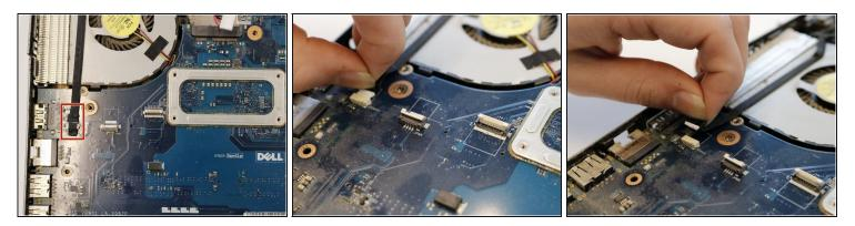
• Unplug the display cable below the fan by pulling the cable straight back.
