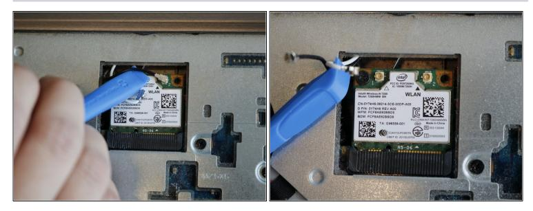
• Use the opening tool to lift both antenna cables upward from the Wi-Fi module.
