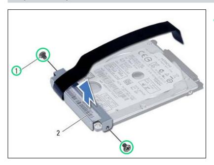
Replace the screws that secure the hard-drive bracket to the hard drive.
