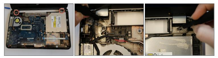
• Remove the two 5mm Phillips #000 screws from the left and right hinges.
