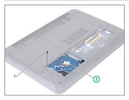
Slide the hard-drive assembly forward to disconnect the harddrive assembly from the system board.
