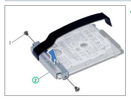
• Lift the hard-drive bracket off the hard drive.
