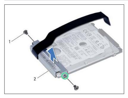
Align the screw holes on the hard-drive bracket with the screw holes on the **NEW** hard drive.
