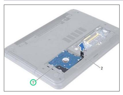
• Slide and place the hard-drive assembly in the hard-drive bay.
