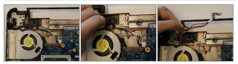
• Remove the DC jack once the display is removed by pulling the cable assembly upwards.
