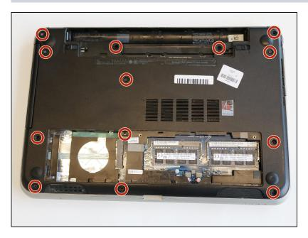
Remove thirteen 5mm Phillips #000 screws from the back cover of the laptop.
