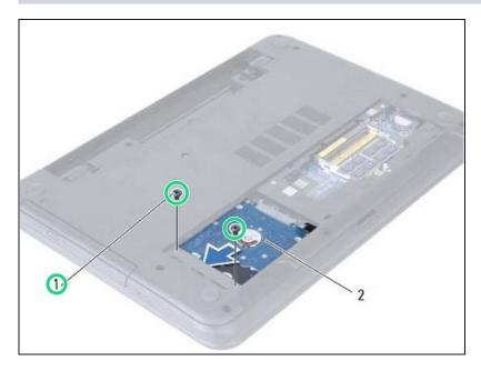
Replace the screws that secure the hard-drive assembly to the computer base.
