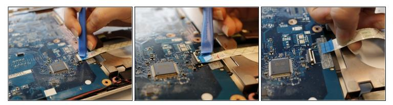
Remove the cable running over the hard drive by using the opening tool to lift the tab and pull back.
