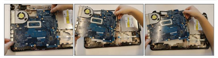
• Remove the motherboard by lifting straight up. Ensure the CD drive is disconnected from the motherboard.
