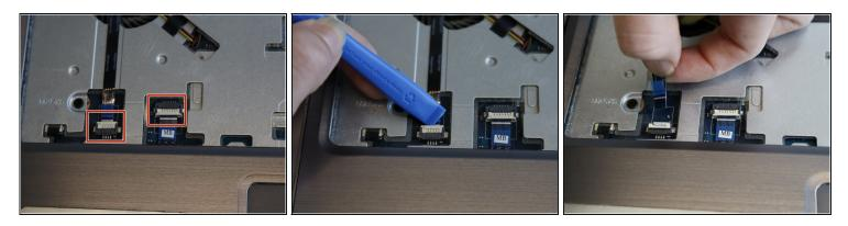
• Use the opening tool to unplug the palm rest cables and slide the cables out.
