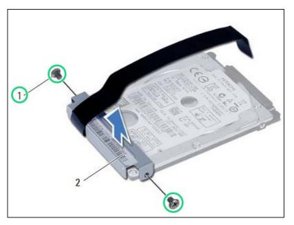
Remove the screws that secure the hard-drive bracket to the hard drive.
