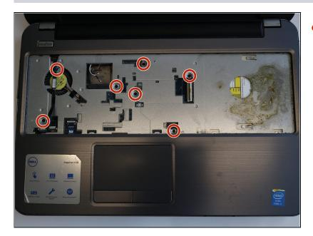
Remove seven 5mm Phillips #000 screws from the midframe.
