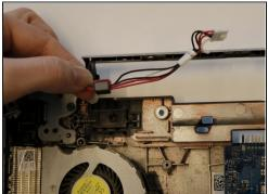
• Remove the DC jack once the display is removed by pulling the cable assembly upwards.
