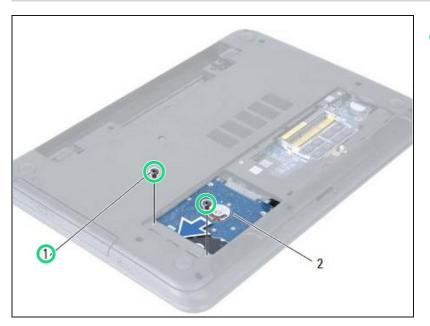
Replace the screws that secure the hard-drive assembly to the computer base.
