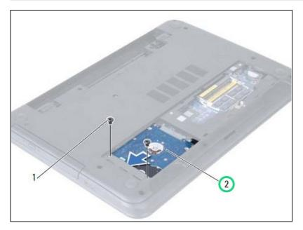
Slide the hard-drive assembly forward to disconnect the harddrive assembly from the system board.
