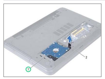
Slide and place the hard-drive assembly in the hard-drive bay.
