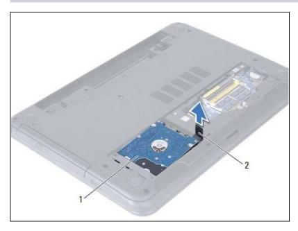
Slide the hard-drive assembly backward to connect the harddrive assembly to the system board.
