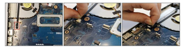
Unplug the display cable below the fan by pulling the cable straight back.
