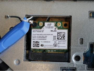
Use the opening tool to lift both antenna cables upward from the Wi-Fi module.
