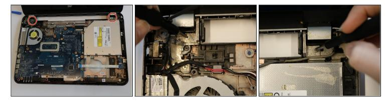
Remove the two 5mm Phillips #000 screws from the left and right hinges.
