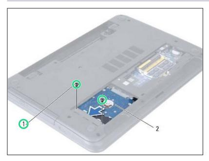
Remove the screws that secure the hard-drive assembly to the computer base.
