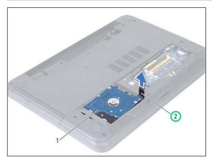
Using the pull-tab, lift the harddrive assembly out of the computer base.
