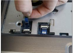
• Use the opening tool to unplug the palm rest cables and slide the cables out.
