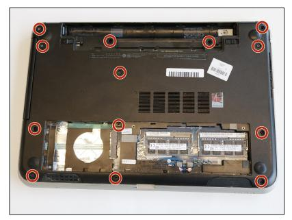
Remove thirteen 5mm Phillips #000 screws from the back cover of the laptop.
