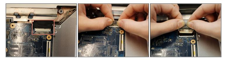
Unplug the display cable located near the right display hinge by lifting the tape and pulling back.
