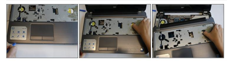
Use the opening tool to lift the edges of the palm rest. Once all of the sides are lifted, pull the palm rest off.
