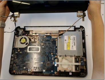
Remove the display assembly by lifting the display from the hinges.
