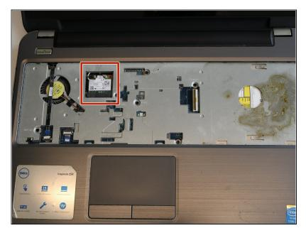
Once the keyboard is removed, the Wi-Fi module will be accessible.
