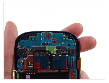
Remove the single 3.0 mm Phillips screw securing the motherboard to the front panel assembly.
