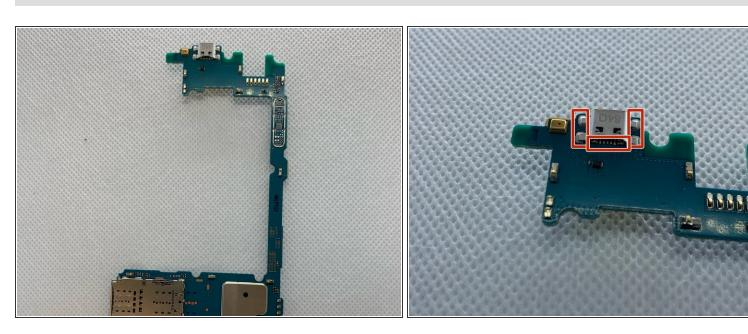
Flip the motherboard over to the backside and use soldering iron to melt the solder on the charging port terminals; use the desoldering wick to remove the solder.
