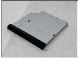
Slide the CD Drive out of the side of the computer by lightly pushing it towards the right side of the laptop.
