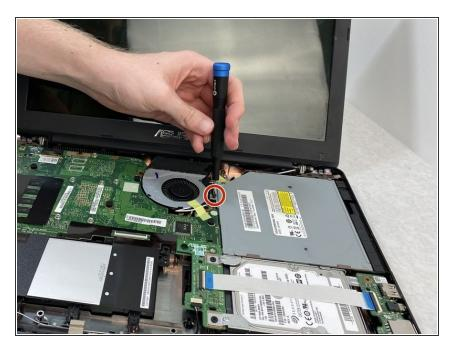
Use the Phillips #000 Screwdriver to unscrew the silver 4 mm screw holding the CD Drive in place.
