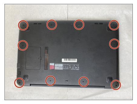
Remove the black 18 mm screws from the back panel of the laptop using the #000 Phillips screwdriver.
