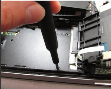
Using a Phillips #0 screwdriver, remove the two 2.0mm Phillips screws underneath the hard drive assembly.
