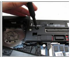
• Using a Philips #0 screwdriver, unscrew the two Phillips screws next to the battery.
