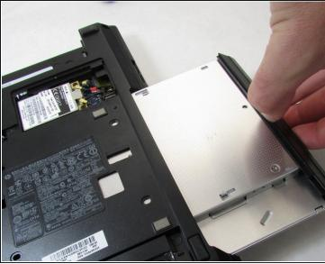
With your fingernail, pry the edge of the optical drive away from the chassis of the laptop and pull it straight out.
