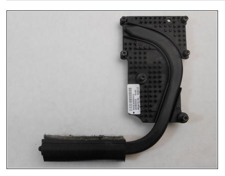
Blow compressed air through the vent from the outside and through the heat sink.
