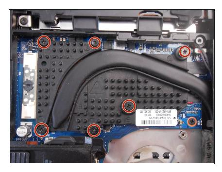
Using a Phillips #0 bit, unscrew the six screws on the heat sink.
