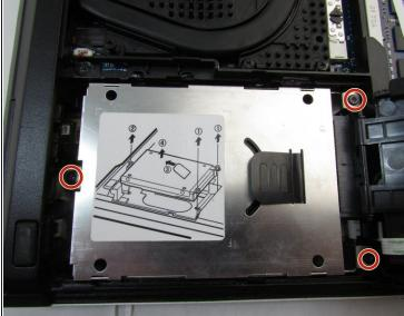
Using a Phillips #0 bit, unscrew the three screws that hold the hard drive assembly in place.
