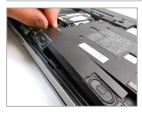
Grasping one corner with two fingers, lift the speaker assembly up and out of the laptop.
