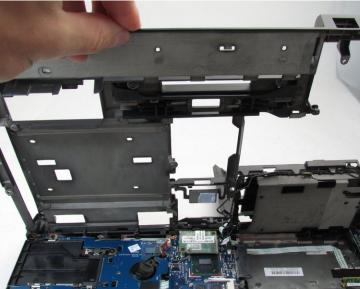
• Lift the chassis up and detach the small connector between the hard drive and heat sink.
