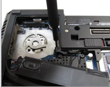
Using a Phillips #0 screwdriver, unscrew the Phillips screw next to the fan assembly.
