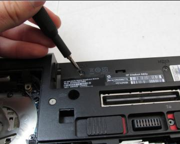
Using a Phillips #0 screwdriver, remove the three 2.0mm Phillips screws underneath the battery.
