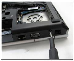
Using a T2 Torx screwdriver, remove the four 8.0mm Torx screws on the back side of the laptop.
