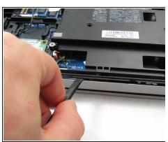
• Using a spudger, work your way around the edge of the laptop popping the plastic chassis up.
