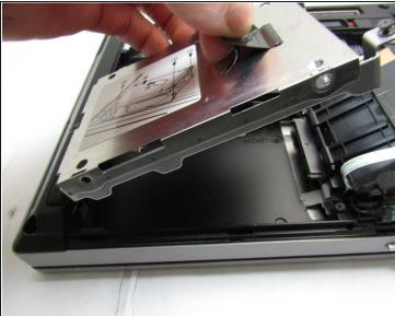
• Remove the silver metal cover by pulling straight up on the black tab.
