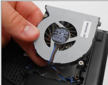
Pull the fan straight up and to the side slightly.
