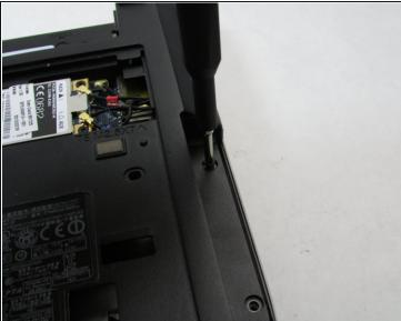
Using a Phillips #0 screwdriver, remove the two 3.0mm Phillips screws to the right of the optical drive slot
