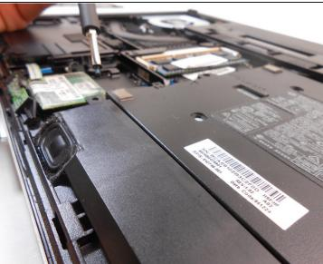
Using a Phillips #0 screwdriver, remove the two 3.0mm screws holding the speaker assembly in place.
