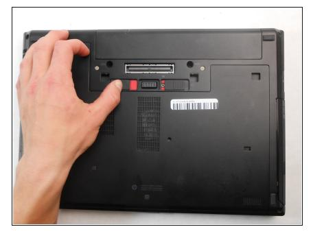
On the back of the computer, slide the left switch towards the outside of the laptop until you hear a click.
