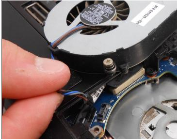
Disconnect the small electrical connector. Pry the edge up with your finger nails or using a small plastic pry tool.
