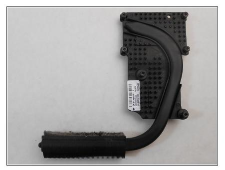
Blow compressed air through the vent from the outside and through the heat sink.
