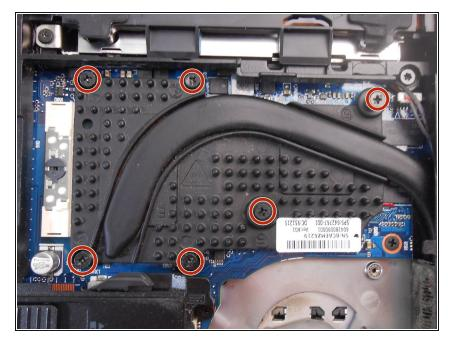
Using a Phillips #0 bit, unscrew the six screws on the heat sink.
