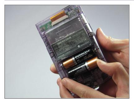
• Remove the batteries from the battery compartment.
