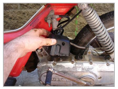
I went to the other side of the bike and removed the carb/oil pump protective cover.
