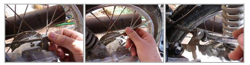
Rear brake gets disconnected next. The cable needs to be free since the brake lever will come off with the rest of the frame.
