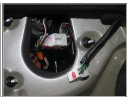
Squeeze down on the top tab of the battery connector. Then, pull the connector out.
