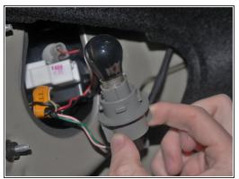
The grey brake light holder is connected to three wires. (Pink, Green, and Black as displayed)
