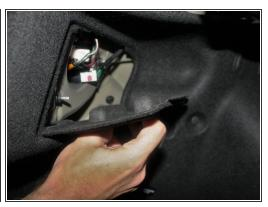
Squeeze and pull back on the felt-like access panel to expose the tail light assembly.
