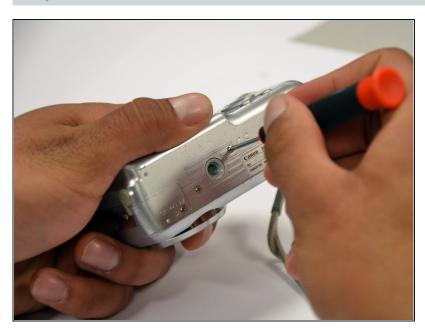
Unscrew the three 2mm Phillips #00 screws that are located on the bottom of the camera.
