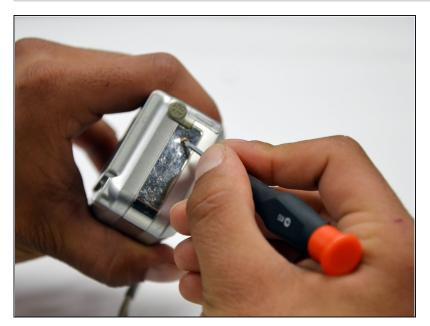
Remove the 4mm Phillips #00 screw that is located on the left side of the camera, if the display screen is facing you.
