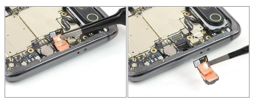
Use a pair of tweezers to lift the front camera out of its recess and remove it.
