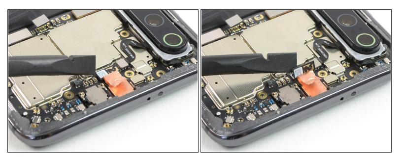
Use the flat end of a spudger to pry up and disconnect the flex cable of the front camera.
