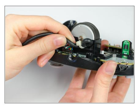
Carefully unhook the cable that is looped around the peg.
