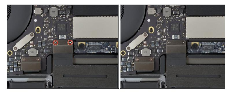
Use a T3 Torx driver to remove the two 1.8 mm screws securing the trackpad cable connector bracket.
