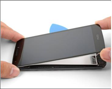
• Lift up the bottom edge of the screen by a few degrees and slice any remaining adhesive.
