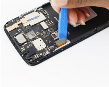
Disconnect the display cable by prying it straight up from the motherboard.
