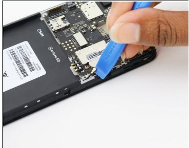
Disconnect the <u>antenna cable</u> by sliding a plastic pry tool or fine tweezers under the wire close to its socket, and then prying straight up.
