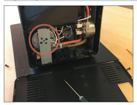
Lift off the back panel, revealing the boiler to the left
