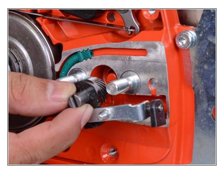
Use your fingers to pull the assembly out of its recess and remove it.
