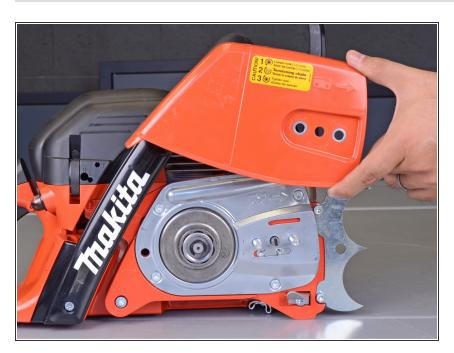
Remove the sprocket guard plate.
