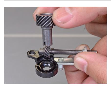
Slide the adjustment screw into the tensioning assembly such that the gears mesh together.
