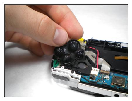
If your button pads did not get removed when removing the front casing, now would be a good time to remove them.
