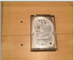
• Slide the hard drive out of its place (this will require a little bit of force)
