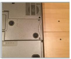
Unscrew the 2 screws holding the Hard Drive in
