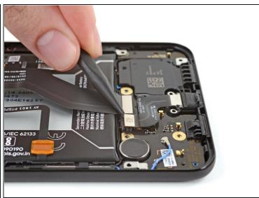
Use the pointy end of a spudger to pry up and disconnect the USB-C port from the lower board.
