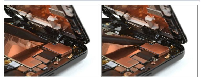
Use a spudger to pry up and detach the proximity sensor cable from the motherboard.
