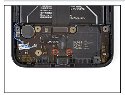
Remove the two T3 screws holding the USB-C port in place.
