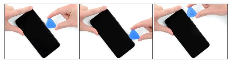
Once the pick is inserted, slide it up and down along the right edge of the phone to cut though the adhesive holding the screen in place.
