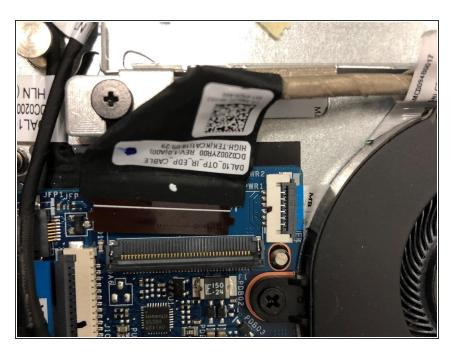
Pull back any tape and gently lift the plastic tab holding the display ribbon in place. Gently pull the ribbon from the socket.
