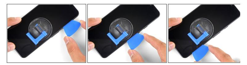
• Slide the pick along the right edge, slicing through the adhesive.
