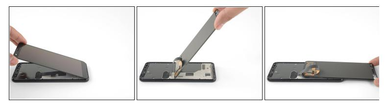
• With all of the adhesives cut, flip the attached screen glass side down and rest it on top of the phone. The screen flex cable should be loosely arched.
