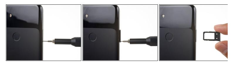
• Insert a SIM eject tool, SIM eject bit, or a paper clip into the SIM tray hole.
