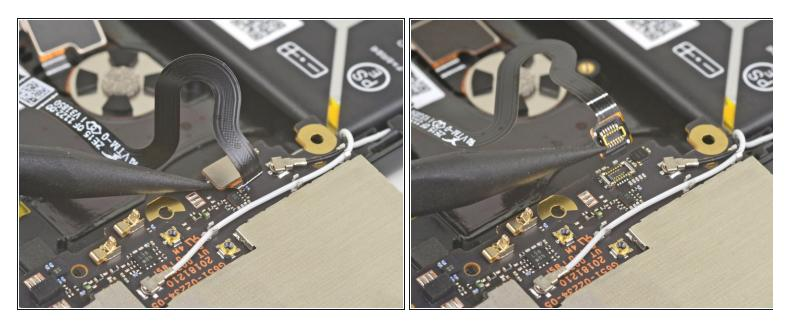
• Use the point of a spudger to pry up and disconnect the fingerprint sensor cable from its motherboard socket.
