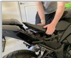
Grab the front section of the seat and slightly lift it up and back to remove it.
