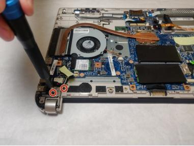
Unscrew 6 screws from the chassis with the Phillips #1 screwdriver.
