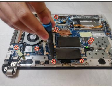
Unscrew 8 screws from the motherboard using the Phillips #1 screwdriver.
