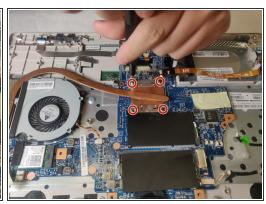
Unscrew screws from the motherboard using the Phillips #1 screwdriver.
