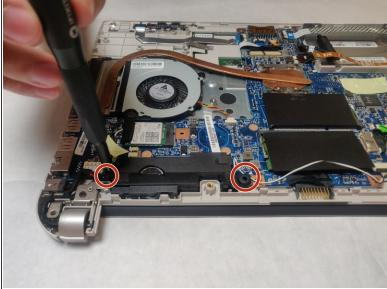
Remove speaker by unscrewing the 4 screws at the side of the speaker with the Phillips #1 screwdriver.
