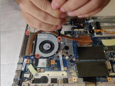
• Unscrew screws from the CPU heat sink using the Phillips #1 screwdriver.
