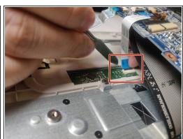
Unscrew the motherboard with the Phillips #1 screwdriver.
