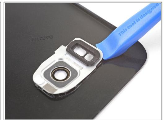
**i** The following four steps show how to remove and transfer the rear bezel. The bezel supports the rear cameras, flash, and the fingerprint sensor (on some models).
