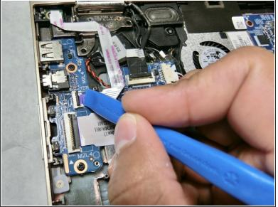
Use the same procedure to disengage the skinnier ribbon cable just above the first: pry up the locking bar of the ZIF connector and slide out the cable.
