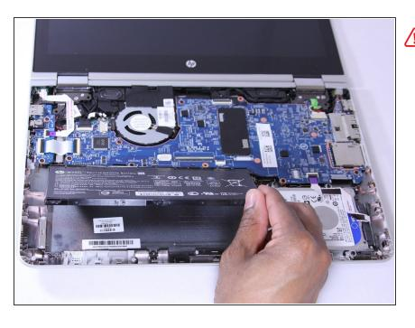
Carefully lift the battery up from lower right corner and disconnect it from the motherboard.
