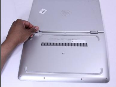
Use a Metal Spudger and remove the rubber foot closet from the bottom of the laptop.
