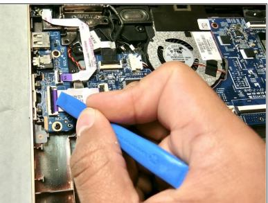
Carefully disconnect the lower ribbon cable by pry the locking bar of the ZIF connector up with a spudger and pulling the cable loose.
