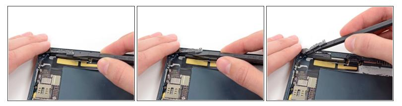
• Use the flat end of a spudger to loosen the foam adhesive holding the antenna to the right speaker.
