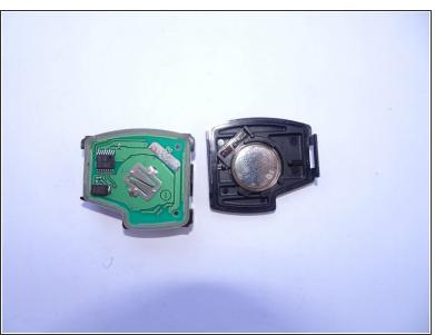
Then you will unclip the middle part. There is one clip on each side of this piece. They are super fragile and can break easily.
