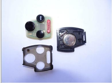
• Then push the buttons from the front side to push out a rubber insert.
