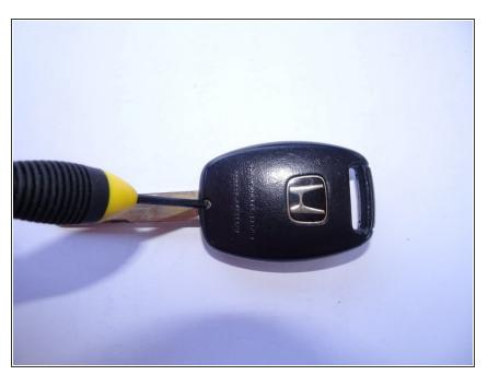
The second step is to take out the little screw on the back side of the key.
