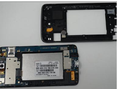
Gently remove the mid-frame using an iFixit opening tool.
