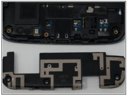
Using an iFixit opening tool, remove the antenna extender located at the bottom.
