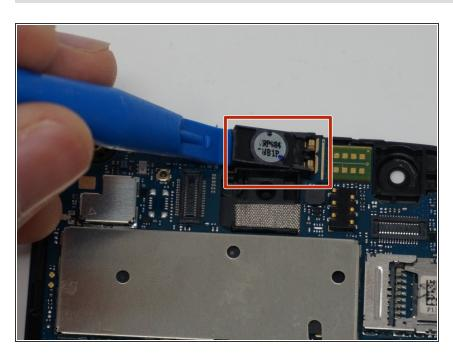
Using an iFixit opening tool, gently pull up the front speaker from its compartment located on the top of the motherboard. To reassemble your device, follow these instructions in reverse order.
