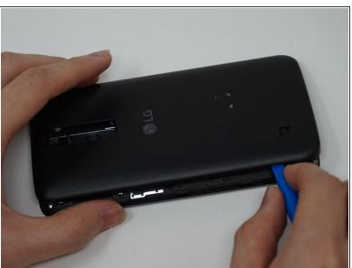
Using an iFixit opening tool, gently pull outward on the cutout on the bottom left corner of the phone to remove the back cover.
